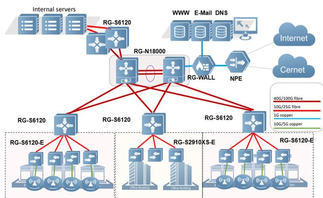
RG-S6120 can be deployed for the access or aggregation of small and medium campus networks. The 10G access ports can be used for high-speed AP access, forming 10G/25G access-to-aggregation and 40G aggregation-to-core high-bandwidth link to meet the users' growing needs.
